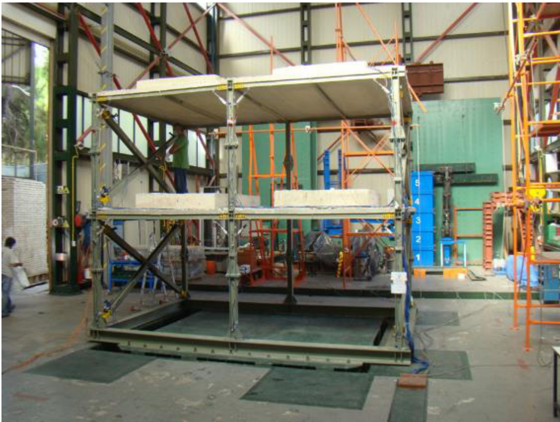
Laboratory for Earthquake Engineering – Earthquake Simulator in front of the Reaction Wall
